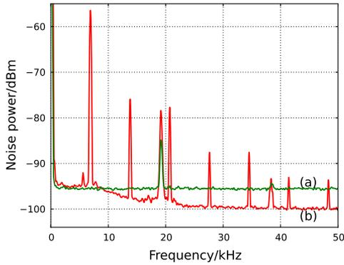
Fig. 4. (Color online) Low-frequency noise power spectrum. (a) SNL and (b) intensity-difference squeezing between the probe and conjugate. 200 Hz RBW.
