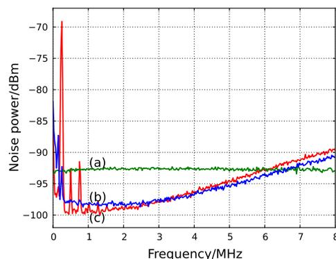
Fig. 2. (Color online) Noise power. (a) SNL, intensity-difference squeezing between the probe and conjugate (b) with and (c) without balancing the intensities of these two beams. 30 kHz RBW and 300 Hz VBW.
