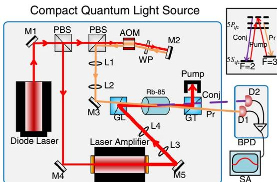
Fig. 1. (Color online) Experimental setup and double- $\Lambda$  scheme of  $^{85}\text{Rb}$  D1 line. M, mirror; L, lens; PBS, polarizing beam splitter; AOM, acoustic-optic modulator; WP, quarter wave plate; GL, Glan-Laser polarizer; GT, Glan-Thompson polarizer; D, detector; BPD, balanced photodetector; SA, spectrum analyzer. Pr, probe, Conj, conjugate.
