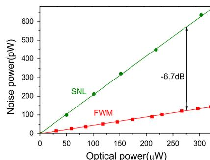
Fig. 3. (Color online) Intensity-difference noise versus total optical power at 635 kHz. Green circles, SNL; red squares, FWM. The ratio of the two slopes is  $-6.7\ \text{dB}$ .
